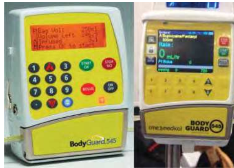
Figure 28.1: Two infusion pumps that are apparently of the same model (photo courtesy of Harold Thimbleby)
