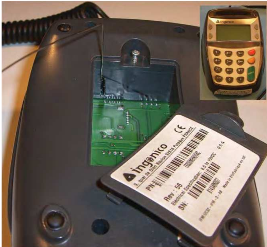
Figure 12.5: A rigid wire is inserted through a hole in the Ingenico's concealed compartment wall to intercept the smartcard data. The front of the device is shown on the top right.
